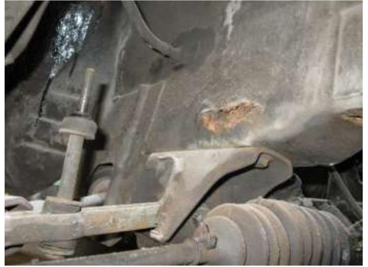
Let the rust repairs commence, with work and other commitments progress on the rust repairs have been slow but with a new rust repair section for the left sub frame rail sourced from Mentiplay Leyland and some other panels cut from some donor cars I have on our block I am making progress.
