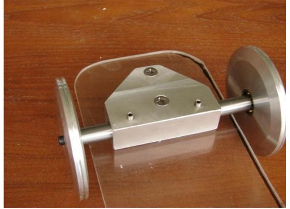
On the right is the front axle which can be adjusted to enable the Racer to run straight.
