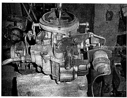
It has an idle solenoid and a float chamber vent. So yours definitely doesn't look like this, but it doesn't run right? Then you have to turn your carby over and look into the throat area just above the throttle when slightly open. There will be a small brass jet sticking out, and above it will be a row of small holes, the idle progression holes. They are DIFFERENT for various versions of the WW, and affect the idle and above idle phases.
