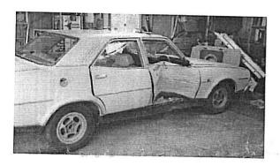
With the P76 the majority of the impact was taken by the driver's door, which entered the cabin enough to touch the steering wheel. The sill was also damaged, and bent inwards approximately 75mm. Miraculously the driver of the P received only minor bruising to his foot. The driver of the Magna was taken from the scene in an ambulance, but fortunately only sustained minor whiplash injuries. The front of the Magna deformed about 400mm as it was designed to.
