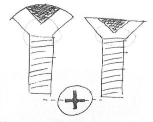
I believe the 'domed' type screw is far superior to the 'flat' type. Originally I thought the previous owner changed the screws for whatever reason. However I recently found the same screws fitted to another P76 a mid 74 Executive. So it would seem there were at least two different types used during manufacture.
