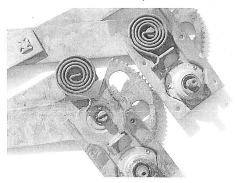
The old right winder has the spring off to show how worn the shaft is. Above is the old left winder with the spring reversed, but not yet hooked on. That only takes a pair of pliers. The spring takes some of the weight of the window, to stop it dropping by itself.
