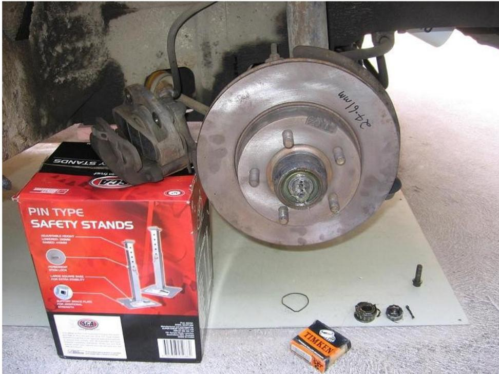
Re-fit the Spring Ring removed from the Old Oil Seal earlier, if you are re-using it, and install the New or Old Seal over the Inner Wheel Bearing, Flat Side Outwards. Tap it in softly with a Wooden Block and Hammer.
