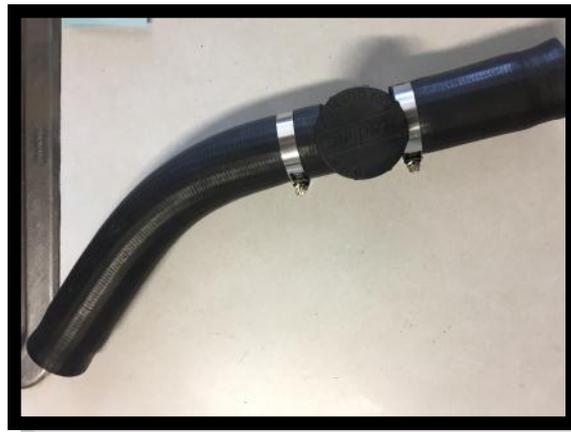
This is a In-Line Radiator filter it's a good thing to have especially if you have had the radiator re-conditioned or flushed also think about a new radiator cap & hi flow thermostat.
