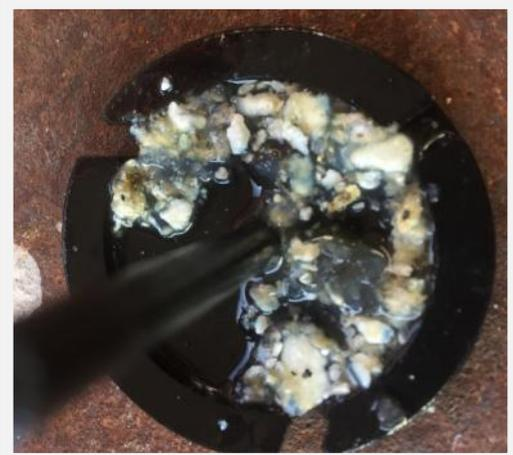
There are 2 filter screens supplied a fine & coarse one this is the fine one you can see that it works & prevents the rubbish before entering the radiator
