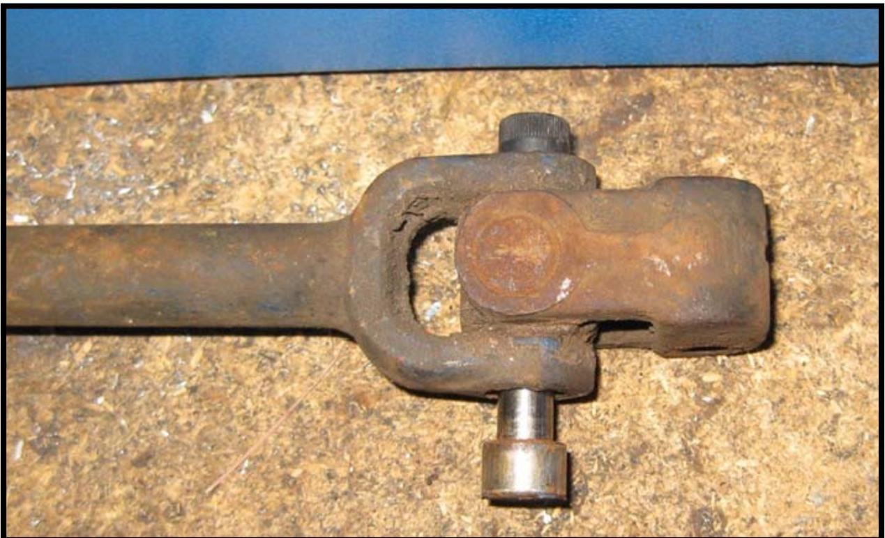
The plastic rings which sit between the block and yoke have protrusions which locate them onto the block and these prevent the joint coming apart once the pin has been removed. Being plastic they can be broken by force or the protrusions can be cut with a razor blade. If the opposite bearing has come out in one piece that side doesn't need to be cut.
