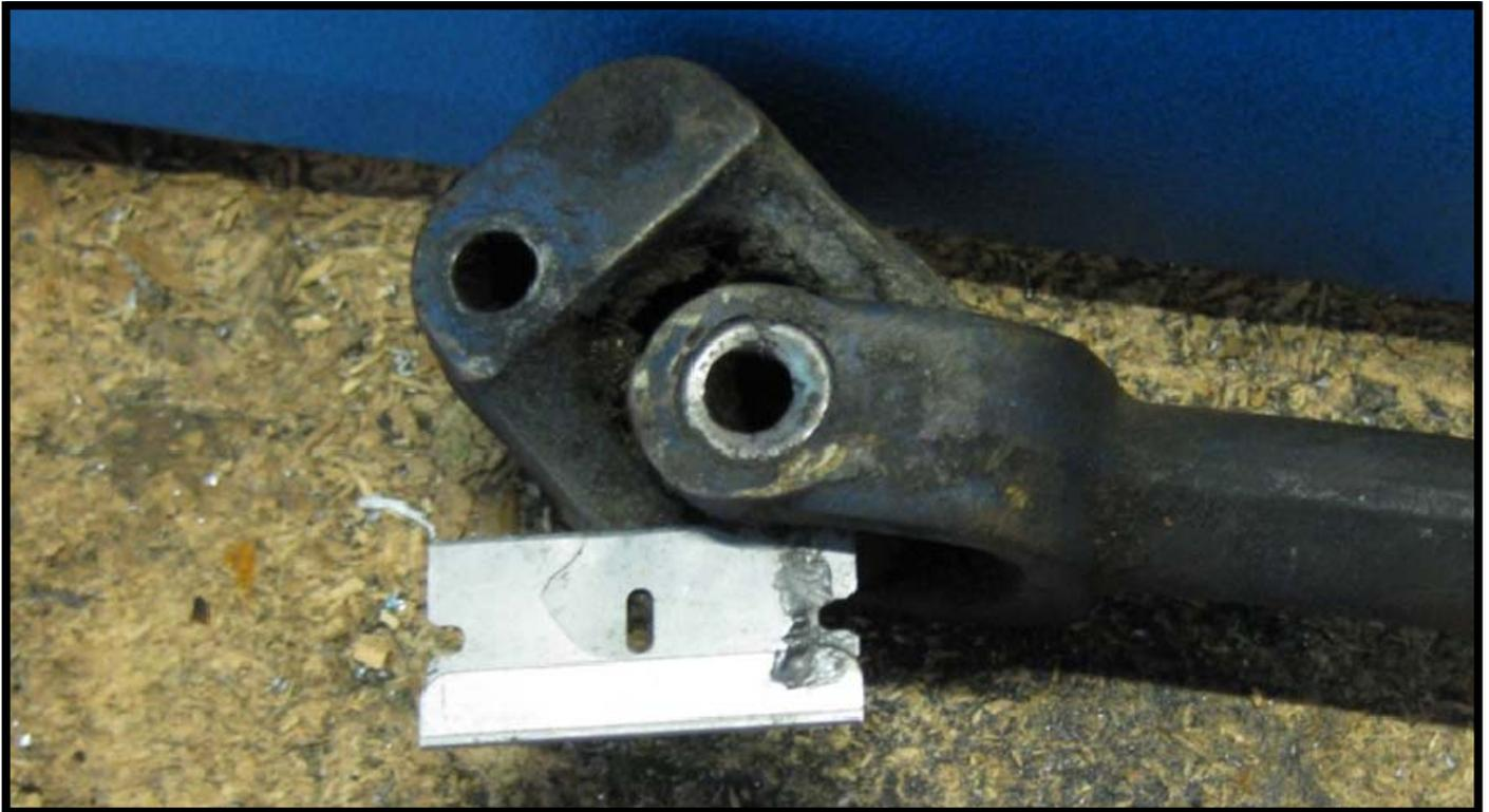
Once the plastic has been cut or broken the block can be withdrawn from the yoke on the shaft. The broken bearing (or bearings) can be removed from the yoke by pressing into the centre of the yoke.
