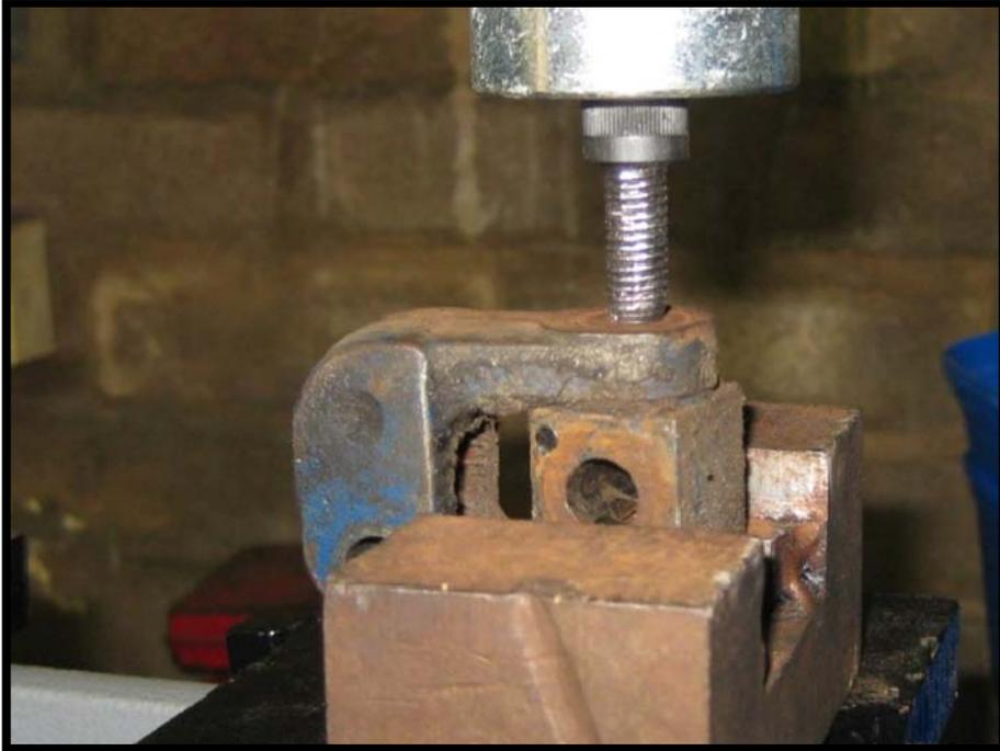
It is likely that the pins removed from the joint will not be suitable for re-use due to wear or corrosion. New pins can be made from "engineer's" dowels which are precision ground, case hardened steel pins. They can be cut and shaped with a grinder by a competent person. Care should be taken not to overheat them as this can change the temper of the metal and affect wear and durability.
