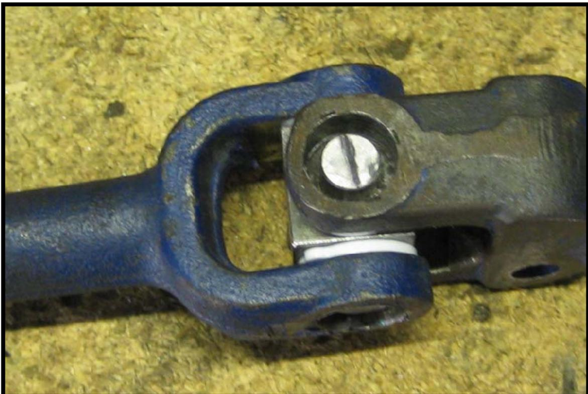
New bearings can now be pressed into place. Apply a small amount of lubricant to the inside of the bearing. I use "Never-Seez" but a waterproof bearing grease would also be suitable. Take care to avoid getting lubricant onto the outside casing of the bearing or the yoke as Loctite is used to retain the new bearing.
